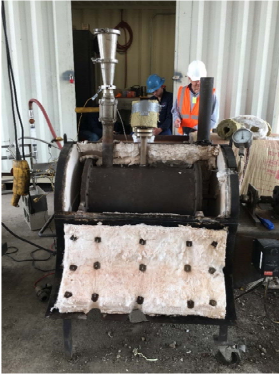
Photo 3: Indirect Thermal Desorption Unit
