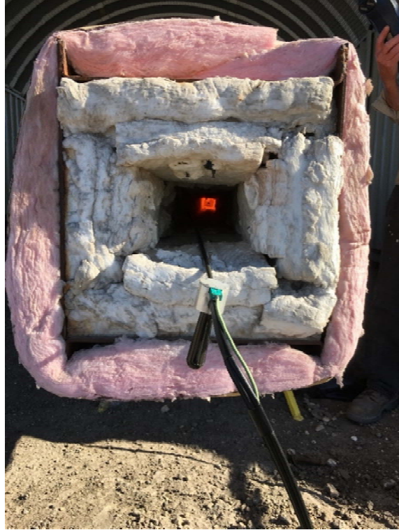
Photo 4: Looking Inside Thermal Oxidizer
