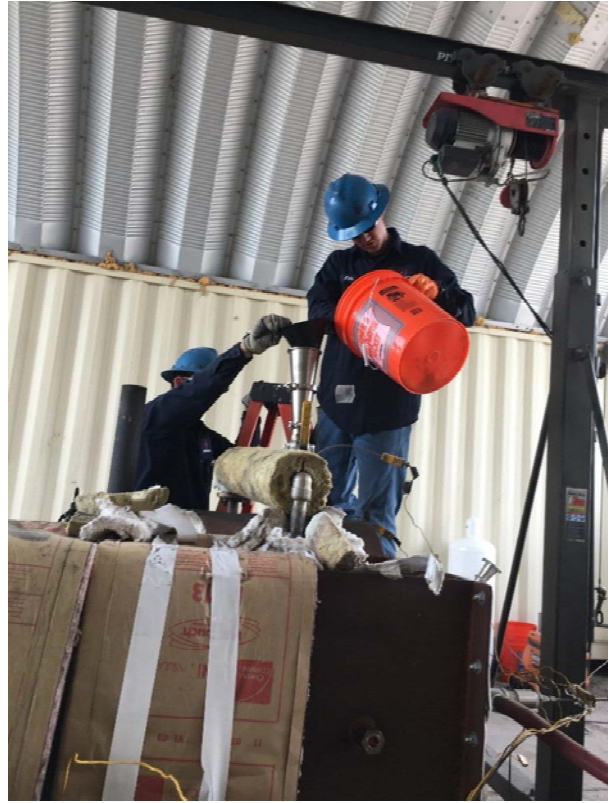
Photo 12 and 13: Feeding Soil to Indirect Thermal Desorption Unit
